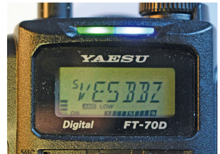
Figure 1 — Display while receiving a C4FM signal from a local System Fusion repeater, indicated by the glowing LEDs at the top.
